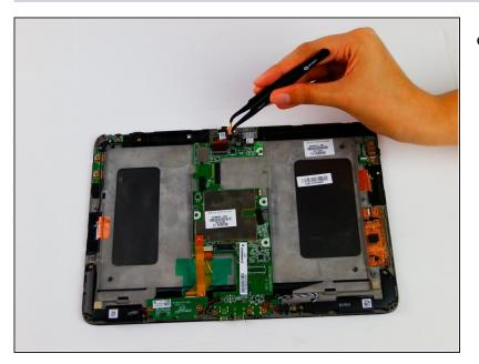
With a pair of <u>tweezers</u>, grab the camera and pull it out of the socket it is in.
