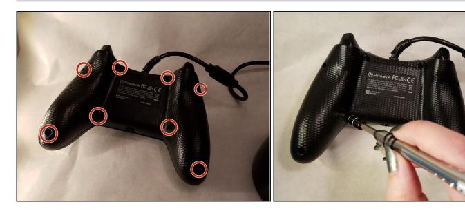
• Disassemble the case by removing the 8 screws, indicated in red on the picture, that hold the back of the case to the front of the case using a J0 screwdriver.
