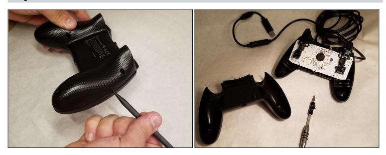
• The case should come apart easily. If not, use a spudger to pry the back from the front of the case.
