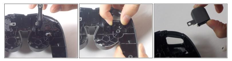
• Finally remove the screws holding in the right and left triggers. It's easiest to hold the trigger together as shown in the third picture. Remove both the left and right trigger, and then you have successfully removed your back panel.
