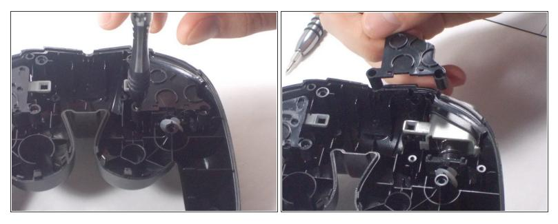
• Remove the screws holding the plastic bumper cover in place and remove it.
