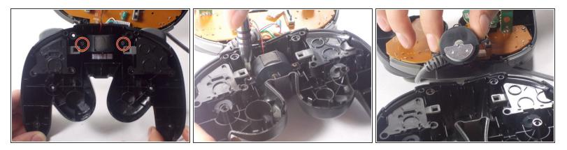
Next, remove the rumble motor by unscrewing the 2 screws connecting it.
