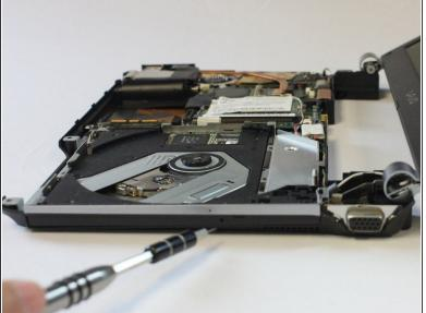
Insert the PH0.8 bit into the pin hole to eject the optical drive.
