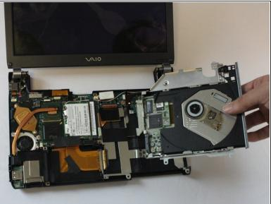
Apply pressure to the ribbon cable, then pick up and pull the optical drive away from the cable.
