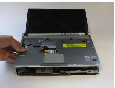
Disconnect the ribbon cable by pulling straight up with your fingers.
