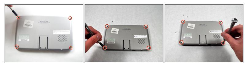
• Unscrew four Phillips #0 screws from the back panel.
