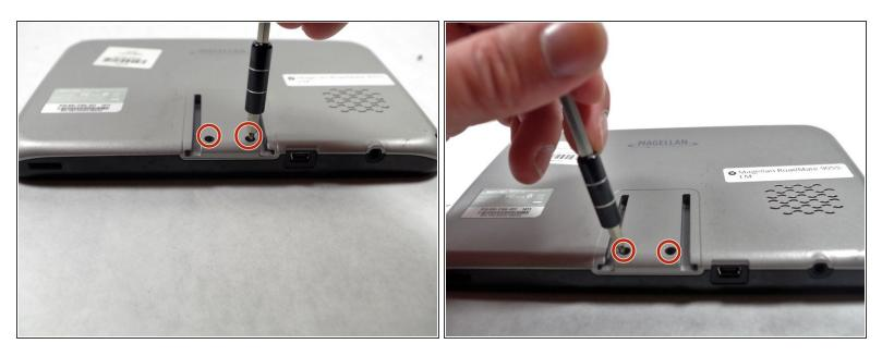
Unscrew two Phillips #0 screws from the back panel.
