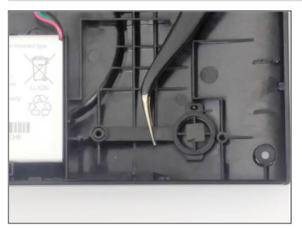
Using tweezers, lift the button out of its socket.
