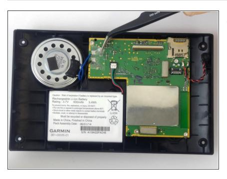
Using tweezers, remove the tape covering the speaker connection to the motherboard.
