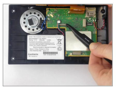
Using the angled tweezers, grip the red, black, and green wires connecting the battery to the motherboard, then gently lift away from the motherboard.
