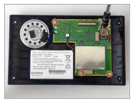
Using the T5 Torx Screwdriver, remove all 4 of the 4.0 mm screws from the motherboard.
