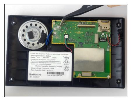
Using tweezers, remove the tape covering the speaker connection to the motherboard.
