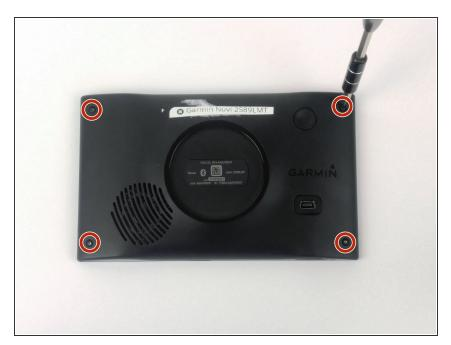
Using the T5 Torx Screwdriver, remove all 4 of the 5.7mm screws from the back of the device.
