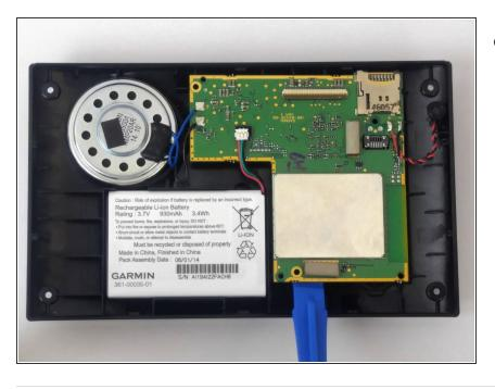
Using the plastic opening tools gently pry the motherboard away from the case.
