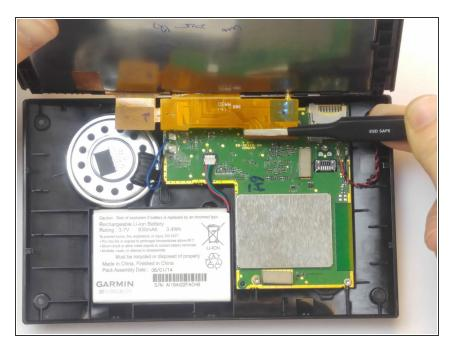
Using the tweezers, gently pull the ribbon wiring near where it connects to the motherboard to disconnect it from the motherboard.
