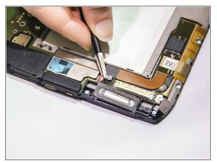
• Using the tweezers, gently pull up the connector off the microphone.
