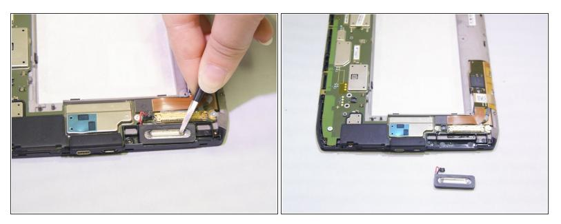
• Once the connector is removed, use the tweezers to pull up the microphone from its plastic socket.
