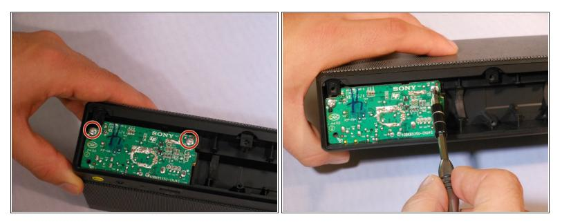
• Using the Phillips #1 screwdriver, remove the two 6mm screws holding the AUX board in place.
