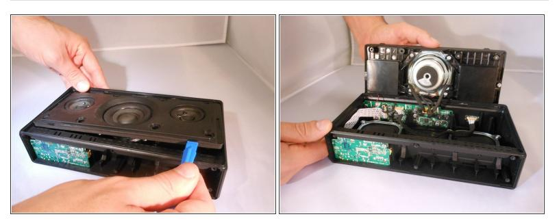
• Using the plastic opening tool, flip open the speaker panel.
