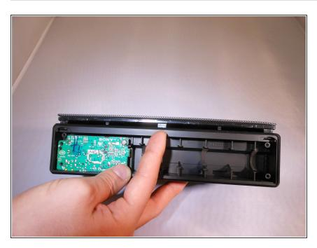
To remove the speaker grill, first push down slightly on the 2 plastic hook tabs to release them, then
