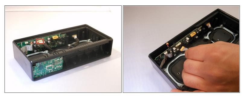
• Unplug the cord connected to the motherboard by squeezing the plastic sides.
