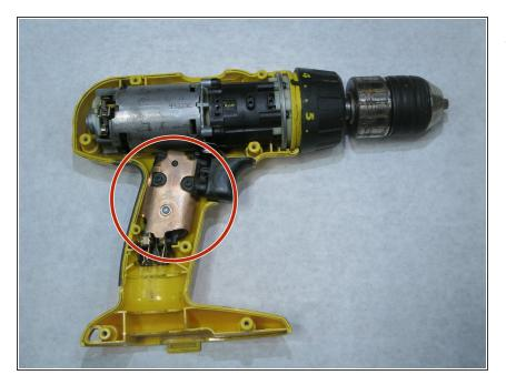
• Carefully remove the trigger pack by lifting the pack straight up.
