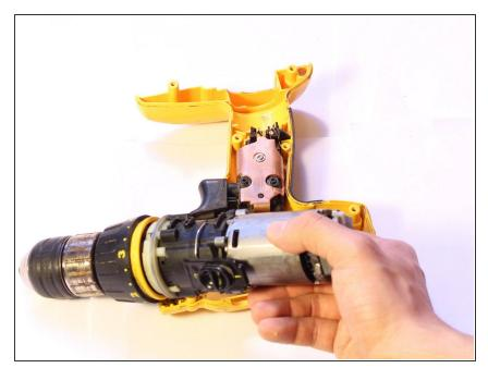
Lift the components out of the casing. These include: motor, gear assembly, trigger assembly and chuck.
