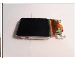
Remove the ribbon cable connecting the monitor and the silver button / dial component. Do this the same way that you did the other ribbon cable.
