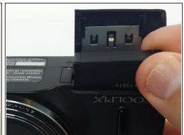
Push the yellow tab inside the battery compartment in the direction of the arrow. This will allow the battery to spring up.
