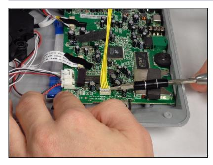
⚠ This guide uses incorrect tools. Use an ESD safe tool, such as a nylon spudger, to complete this step.
