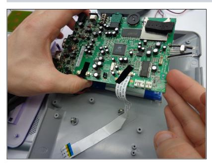
• Lift motherboard to expose battery
