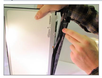
Pull the black tape that is attached to the frame off of the screen
