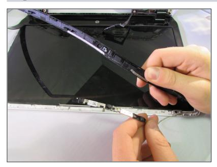
⚠ When prying the screen frame off be careful around the top edge as your webcam will be there. It is a safe idea to move it out of the way like am I doing now.
