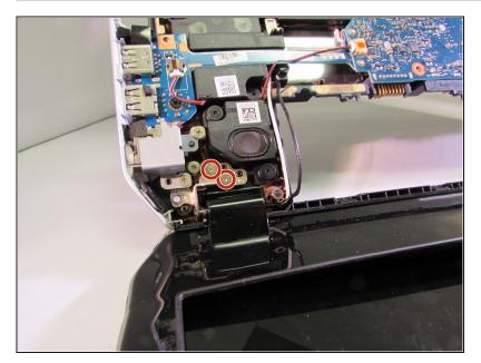
Using a Phillps #1, remove the two 5.6mm silver screws from the base of the first hinge.
