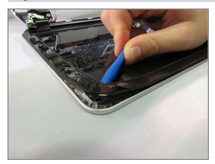
Using a plastic opening tool, carefully start prying the frame of the screen up
