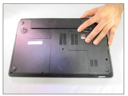
• Slide the release mechanism to the left to release the battery.
