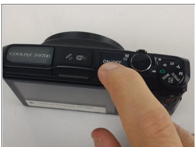
Press the ON/OFF button to power off the S9700.
