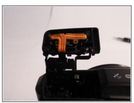
Using your fingers or plastic opening tool, remove the back half from the front half of the flash housing. The front half will stay on.
