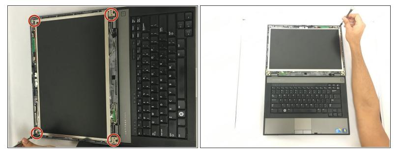
• Use the Phillips screwdriver to remove the screws from corners around the screen.
