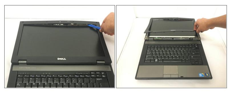
Using a plastic opening tool, pry the bezel away from the screen.
