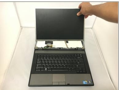
Release the screen by pulling up and out.
