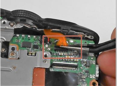
Gently detach the flex ribbon with your tweezers before removing the front plate.
