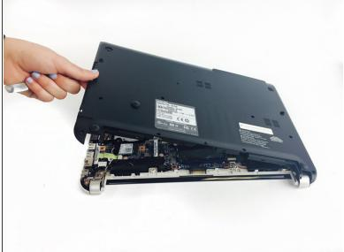
• Using a spudger, poke the white tabs in by the battery until you hear a click.
