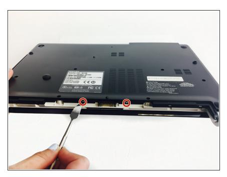
Using a spudger, poke the white tabs in by the battery until you hear a click.
