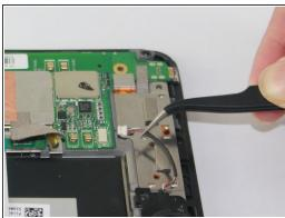
Use tweezers to grab the speaker cable near the white plug and pull to disconnect it.
