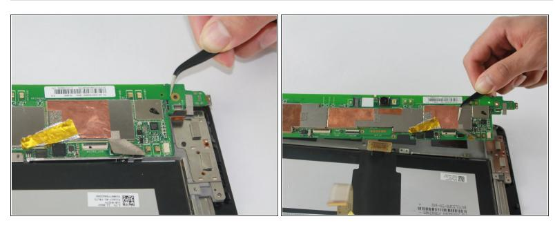
Slide the tweezers under the motherboard and lift up to remove the motherboard.
