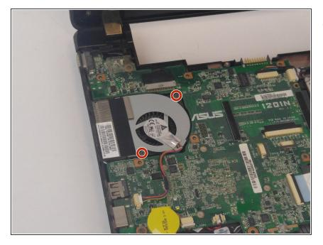
Remove the two 4.6 mm screws from the cover plate using the J0 Phillips head screwdriver.
