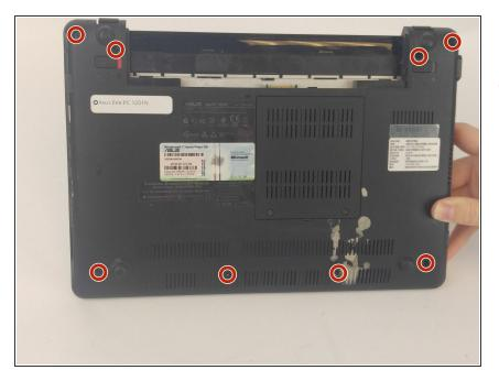
Remove the eight 6.5mm screws using the J0 Phillips head screwdriver from back of the netbook.
