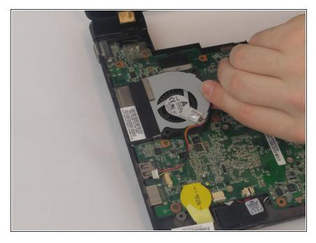
• Lift up and remove the fan.
