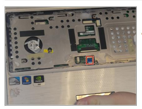
Pull the blue tab for the touchpad connector before removing the cover plate completely.
