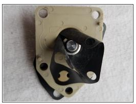
Reinstall the new diaphragm in the intermediate plate.
