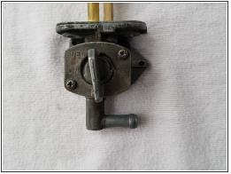
Thread the spring washer and the cover plate into the actuator and build it into the base body.
