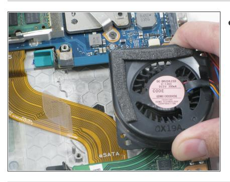
You can now safely remove the fan completely and replace it with your replacement fan.
