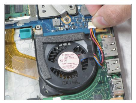
Disconnect the fan's power cables from the motherboard by gently pulling the white connector towards the fan and away from the motherboard.
