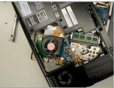
• The back cover of the laptop can now be removed by gently lifting its edges with your hands. Avoid abrupt removal of the back cover because it is attached internally. Move the cover to the side and the fan will now be visible.
