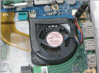
Remove the two 50mm screws holding down the fan using a Phillips #00 screwdriver.
