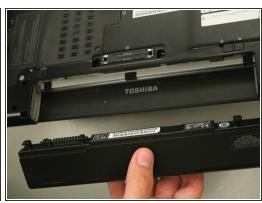
Hold the next lock in the unlock position. Simultaneously pull the battery towards you.
