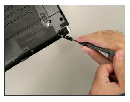
Begin by removing 14 70mm screws from the back cover of the laptop using a Phillips #00 Screwdriver. Do not attempt to remove the back cover just yet though.
