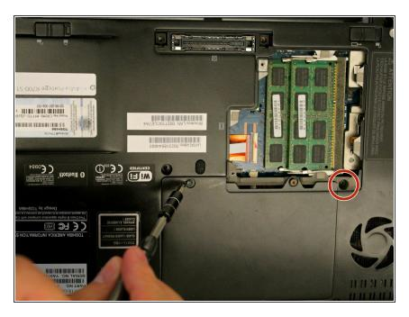
Next, unscrew 2 40mm screws using a Phillips #00 Screwdriver. The back cover will now be able to be removed with greater ease. Note the previously covered 70mm screw illustrated by a red circle on the image.
