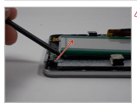
★ Knowing the location the ribbon cable, use plastic spudger to pry off battery.
