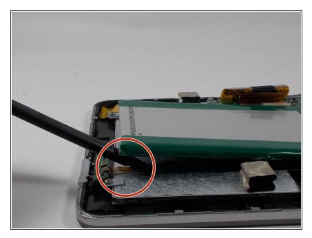
There is a small ribbon cable located under the battery. running from the volume buttons underneath the batter to main logic board.
