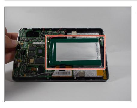
Locate battery. The battery is the silver coated square shaped device on the top of the motherboard.
