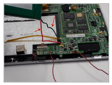
After the battery is free from the logic board, find the positive and negative wires that connect the battery to the motherboard
