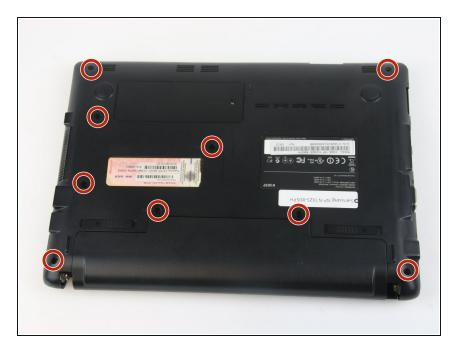
Using a Phillips #0 screwdriver, remove the nine 6.5 mm screws.
