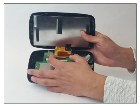
Once the two covers are separated, use your fingers, to gently disconnect the wires that are connected to the motherboard from the back cover.
