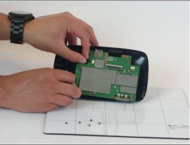
Separate the motherboard from the front cover, you must disconnect the wires connecting the two.
