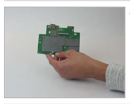
The motherboard is now disconnected from the front assembly
