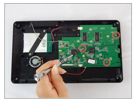
Use a J1 Phillips screwdriver to remove the three 6.1 mm screws on the motherboard.
