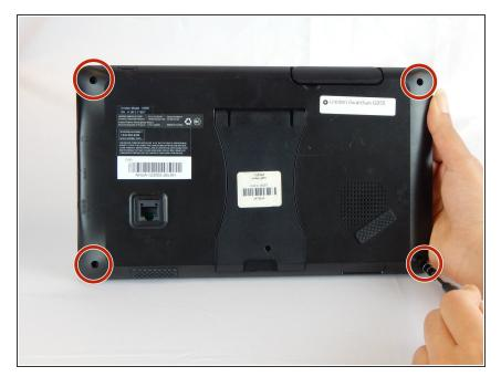
Use a J1 Phillips screwdriver to remove the four 6.1 mm screws at the back of the monitor.
