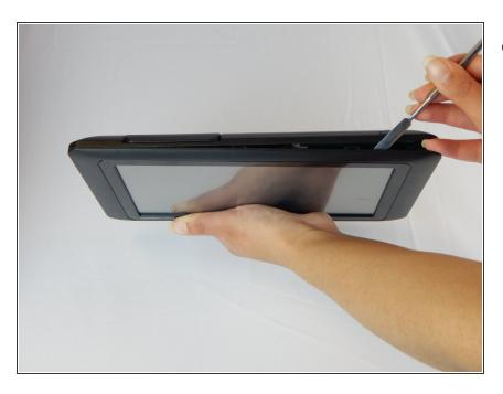
Use a metal spudger or an opening tool to pry open the device.
