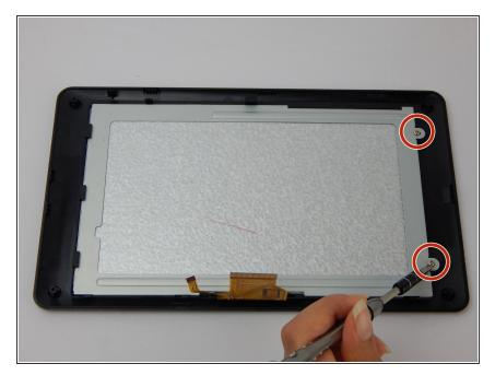
Use a J1 Phillips screwdriver to remove the two 6.1 mm screws.
