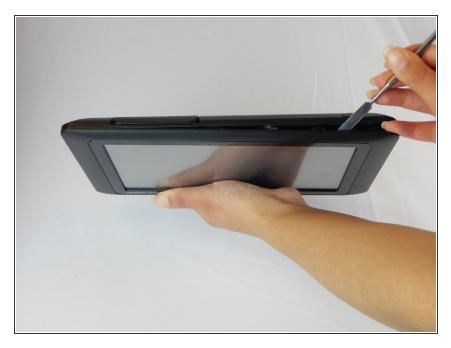
Use metal spudger or an opening tool to pry open the device.
