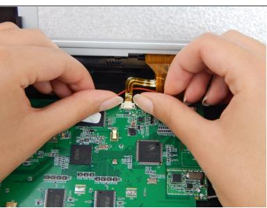
In both pictures, disconnect the zero insertion force (ZIF) connector from the motherboard using your fingernail by sliding up on the male end of the connector to loosen it.
