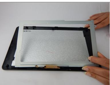
Apply pressure to metal casing and slide off.
