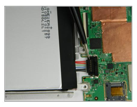
Make sure that the battery is disconnected from the motherboard by unplugging the ribbon cables.
