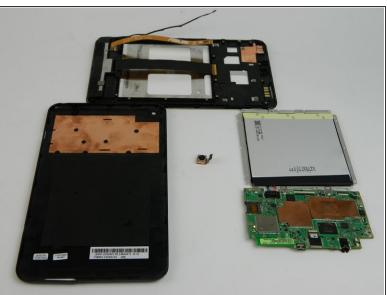
Flip Motherboard assembly over and pick out camera. Now the Front Facing camera can be replaced.
