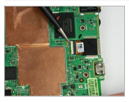
In the middle of the Motherboard there will be a little ribbon cable (white tab must be lifted to removed cable.)
