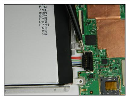
Make sure that the battery is disconnected from the motherboard by unplugging the ribbon cables.
