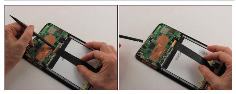
• Use the flat end of the nylon spudger to flip up the retaining flap of the ZIF connector holding the black motherboard ribbon cable in place.
