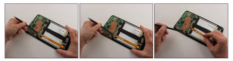
• Use the flat end of the nylon spudger to flip up the retaining flap of the Zero Insertion Force (ZIF) connector holding the orange motherboard ribbon cable in place.
