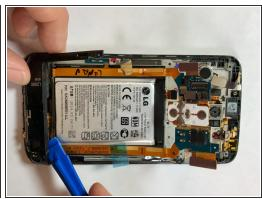
The bottom inside panel should pry back easily after you take out the screws. Again, if the panel does not pull off easily, you may have missed a screw.
