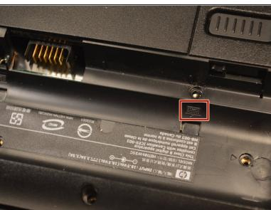
• Locate the three screws for the keyboard by finding the small keyboard picture, remove these screws and flip the laptop back over.
