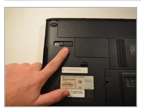
Slide the battery release bar to the left, this should release the battery so you can then remove it.
