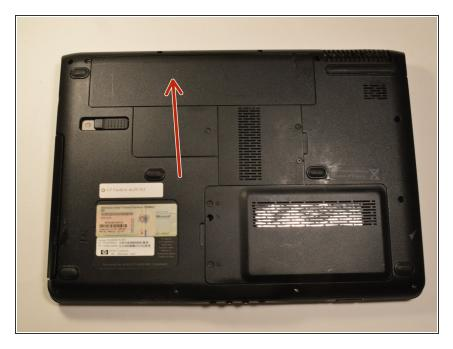
Locate battery on the bottom of the laptop.
