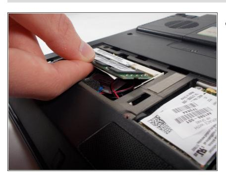
Remove the old RAM by lifting it upwards, then pulling.
