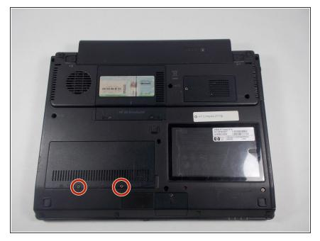
Flip the device over so the back panel is facing upwards. Locate the RAM plate cover towards the left side of the laptop. There will be two screws located on the panel.
