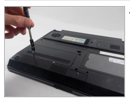
Remove both screws holding the RAM cover plate in place using your Phillips Screwdriver.
