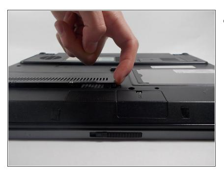
Remove the cover plate by lifting upwards once screws are removed.
