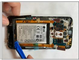
• The bottom inside panel should pry back easily after you take out the screws. Again, if the panel does not pull off easily, you may have missed a screw.
