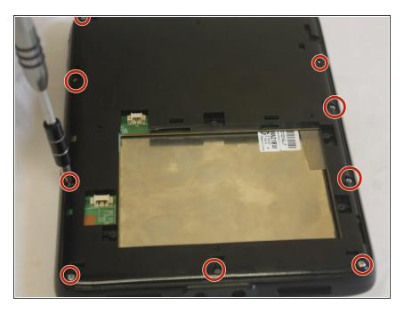
Remove the twelve screws in the cover with a Phillips #0 screwdriver.
