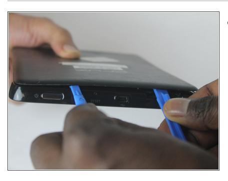
Insert a second opening tool into the space created by the first opening tool.
