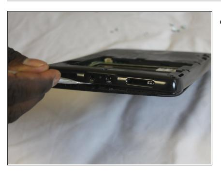
Move the spudger around the face to release the clips attached to the tablet base.
