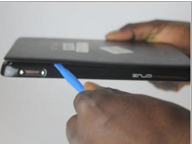
Slide the opening tool across the back plate to disconnect the clips joining the plate to the tablet.
