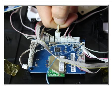
Follow the cord for the circuit board from the whammy bar, and using your hands pull it out of the main circuit board.
