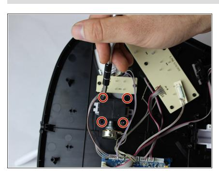
Using a size J1 philips head screwdriver, remove the four black 5 mm screws (circled in red) from the
