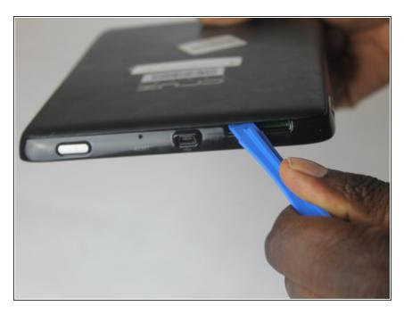
Insert the plastic iFixit opening tool into the SD port. Orient the iFixit opening tool so that the edge faces the rear panel.
