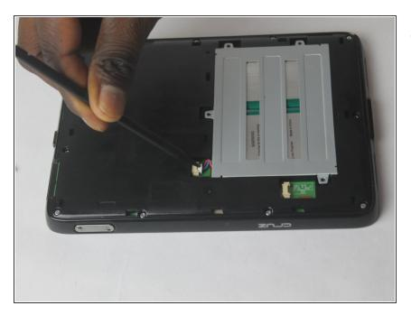
Disconnect the battery using the spudger.
