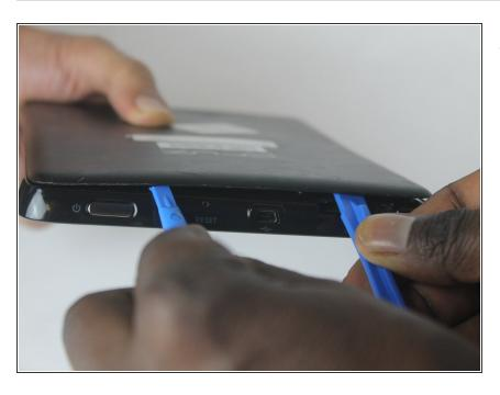
Use the iFixit opening tools to pry open a gap between the tablet and rear panel.
