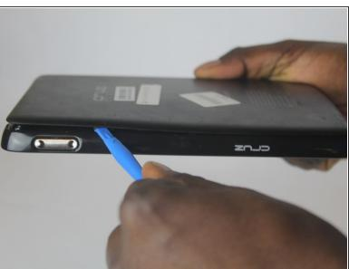
Move the small tool opener around the rear panel to free the 12 clips.
