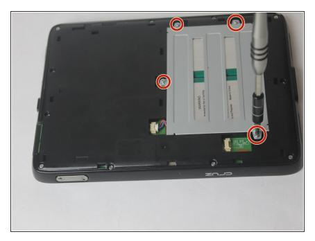
Remove the four screws in the metal battery housing using the Phillips #0 screwdriver.
