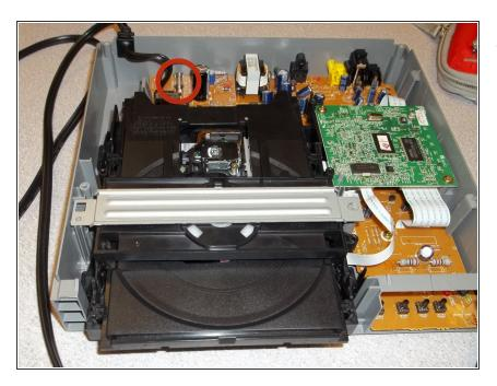
Now that the device is open, you can check for any blown fuses that may need to be replaced.
