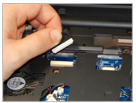
• Unhook the display connector wire.
