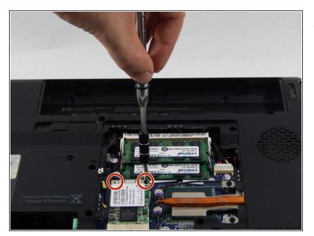
Locate and unscrew the two Phillips head 3 mm screws on the wireless card.
