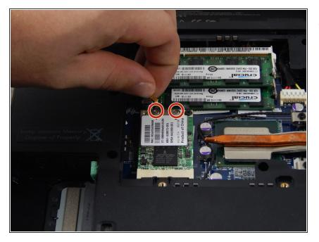
Unhook the two wires connecting to the wireless card by gently pulling them out.
