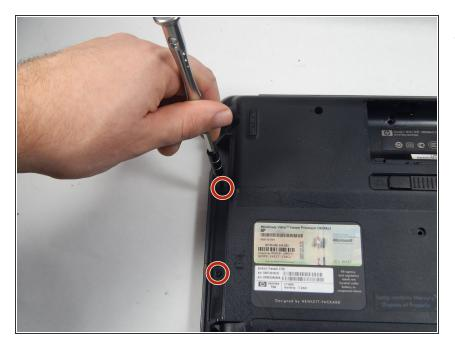
Use the PH0 screwdriver to remove the two 3 mm Phillips head screws in the disk drive port.
