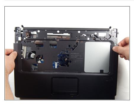
• Remove the cover by lifting it.
