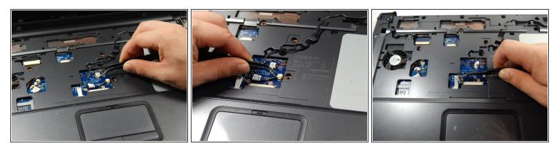
• Unplug the remaining wires using the tweezers.
