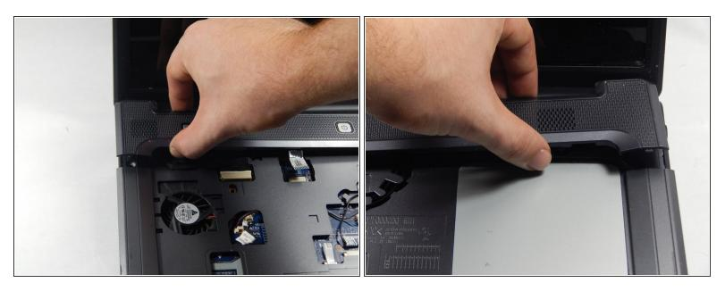
• Press and hold the lock to pop the panel piece above the keyboard and pull up to remove it.
