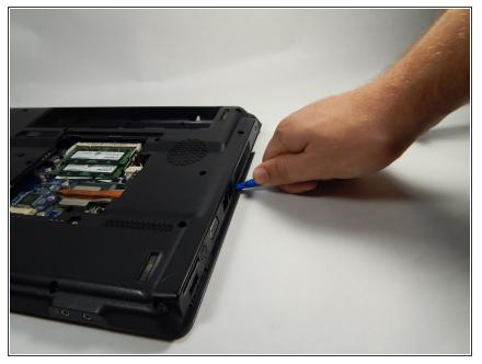
• Use the plastic opening tool to pry up all sides of the device cover.
