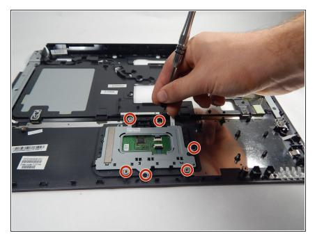
Use the PH0 screwdriver to remove the six 1 mm Phillips head screws surrounding the touchpad
