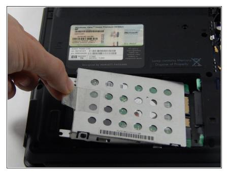
• Remove the hard drive by pulling on the plastic tab and lifting upward.
