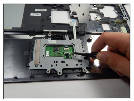
• Use the tweezers to remove the touchpad wire connection.
