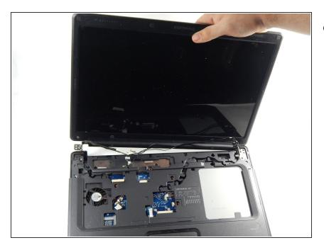
• Gently disconnect the display by pulling it upwards.
