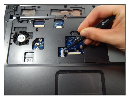
• Disconnect the touchpad connection using the tweezers.
