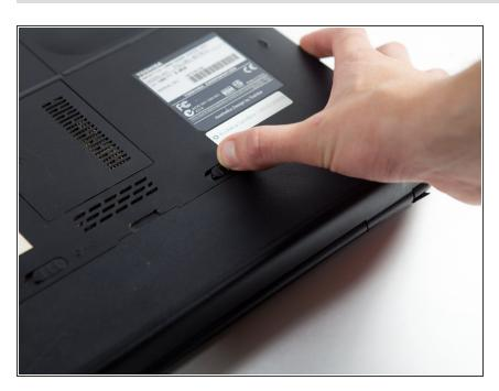
Set the right-hand switch near the battery into the unlock position (move switch from left to right).
