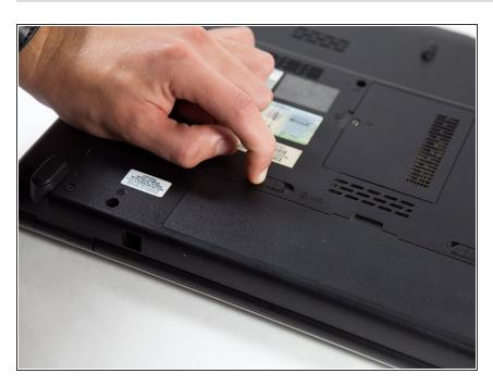
Set and hold the left hand switch near the battery into its unlock position (move switch from right to left).
