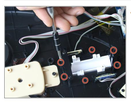
Using a size J1 head screwdriver, remove the six black 5 mm screws (circled in red) from the back of the strum button component.
