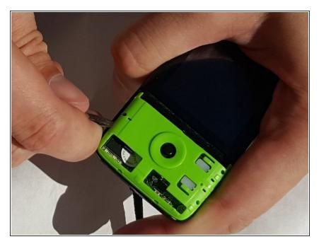
Find the groove around the outside of the green section. Use an ESD safe spudger to slowly lift the plastic panel up.
