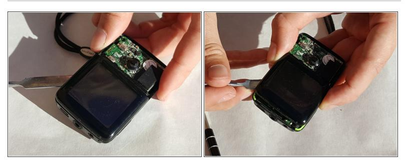
After removing the green section, find the groove around the display. Insert a ESD safe spudger and carefully lift the display.
