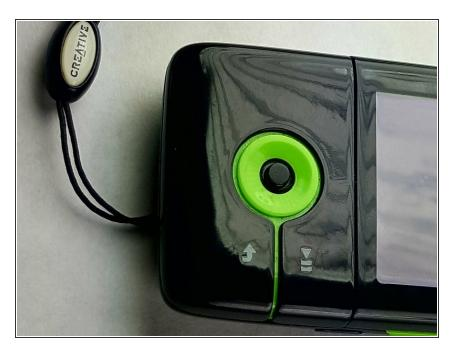
Find the grooves around the buttons on the front and carefully remove the panel. This can be done without the use of any tools.
