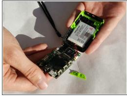
Pull up on the motherboard and display. It is glued to the base so it will require a little force. Be careful though, as the board is fragile.
