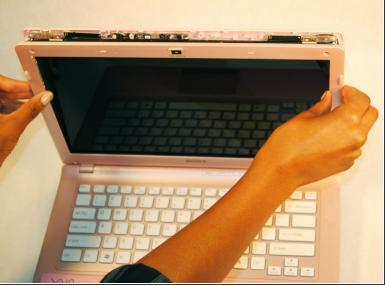
After all of the screws are removed, gently pull on the frame to remove it.
