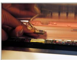
Detach the wire that is connected to the LCD screen by grabbing back of connector and sliding it out.
