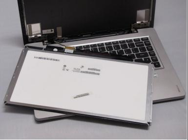
• Once the four screws are removed, gently rest the screen facedown on the keyboard.
