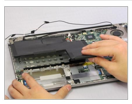
Remove the battery by lifting up and away from device.
