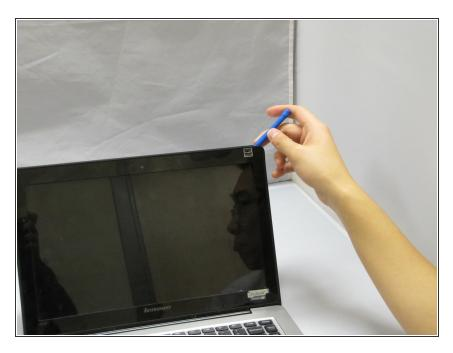
Insert opening tool between the frame and the back panel of the screen.
