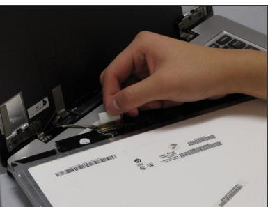
Peel back the white tape, revealing the power connection.
