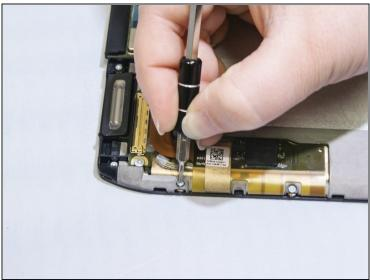
• Remove thirteen 2.55mm Torx #4 screws with Torx T4 screwdriver.
