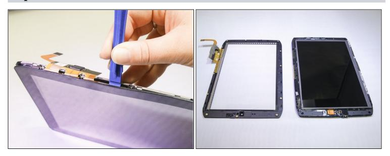
• Use a plastic opening tool to gradually separate the screen from the device.
