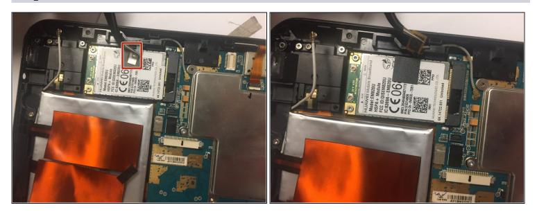
• Using <u>tweezers</u>, remove the tape connected to the GSM module.
