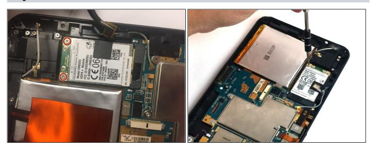
• Remove the two 3mm screws securing the GSM module. Use the Torx screwdriver.
