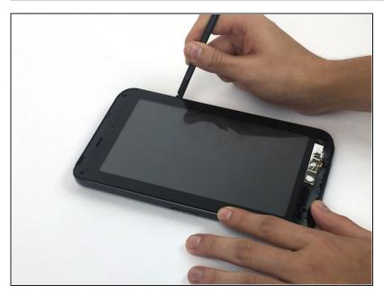
Use the spudger to go along the edges of the device and pop out the latches securing the display to the case.
