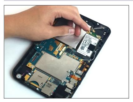
Disconnect the GSM module by lifting the module up, out of the case.
