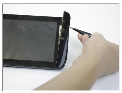
• Remove the button cover by lifting the cover away from the tablet.
