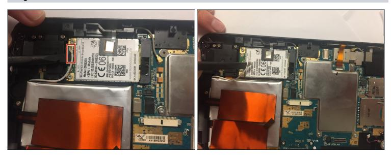
With the spudger, disconnect the antenna cable located on the module.
