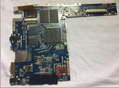
Carefully lift and remove the motherboard from the device housing.
