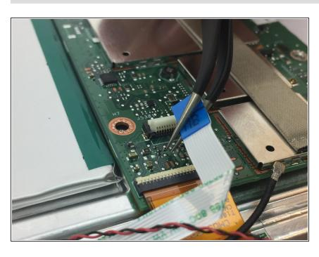
With tweezers, gently flip the white clip up that is holding the white ribbon cable down. Pull the base of
