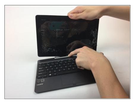
Detach the screen from the keyboard using the silver button and pulling the screen in the upwards direction.
