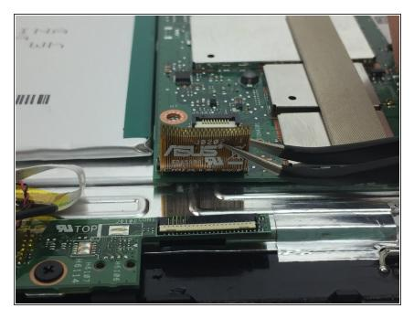
Disconnect the bottom orange ribbon cable with tweezers by pulling it away from the edge of the device.
