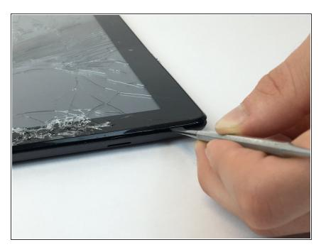
Pry the plastic backing off of the tablet using the plastic spudger, releasing all interior clips.
