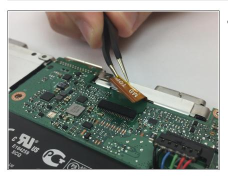
Gently pry the orange ribbon cable that is near the battery cable upwards with tweezers.
