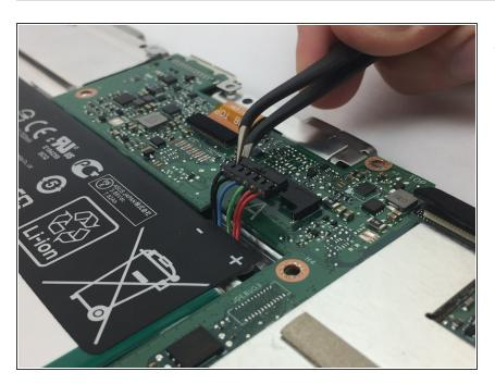
Detach the battery cable by steadily pulling it away from the motherboard with angled tweezers.
