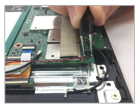
Use tweezers to detach the black and red twisted pair cable from its connection to the motherboard.
