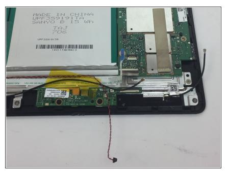
Verify that cables are no longer attached to the motherboard.
